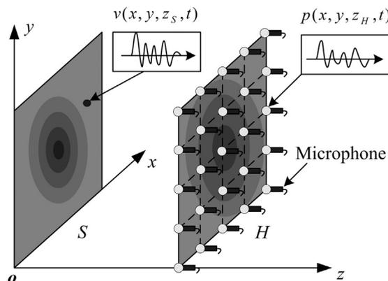
Fig. 1. Geometry of the source plane  $S$ , the hologram plane  $H$ , and the microphone array.
