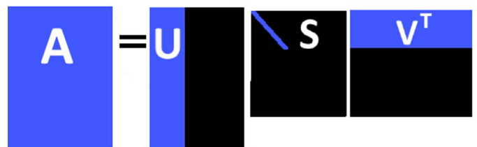
Fig. 1. Decomposition of input matrix \mathbf{A} into diagonal matrix of singular values \mathbf{S} and matrices of left and right singular vectors. Light color illustrates low-rank approximation.
