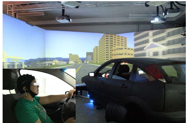
Fig. 1. BJTU driving simulator and electrode cap on driver.
