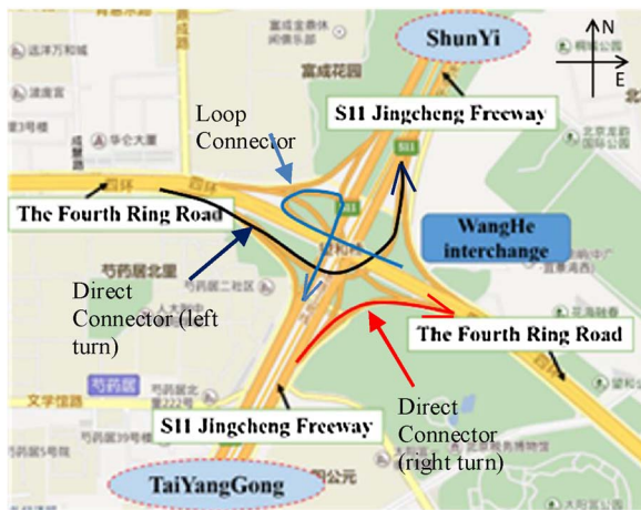
Fig. 1. Types of connectors in an interchange in Beijing. (For interpretation of the references to colour in the text, the reader is referred to the web version of this article.)
