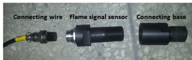
Fig. 2. Photo of the flame signal sensor.
