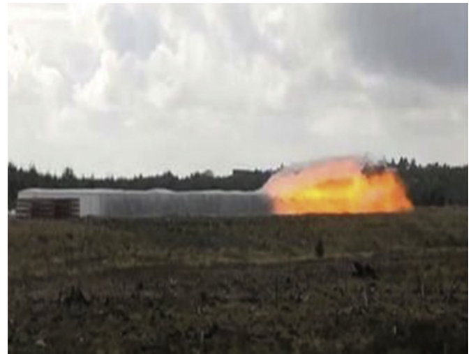
Fig. 1. A flame acceleration experiment in a 100 m long rig congested by pine trees. Deflagrative flame propagation is visible from right to left.
