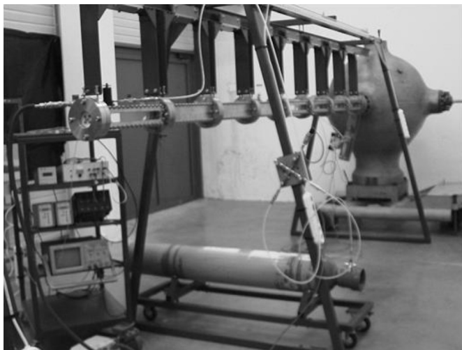
Fig. 1. Equipment used by Kerampran (2000), 4 m long tube, 40 mm wide, square cross section.
