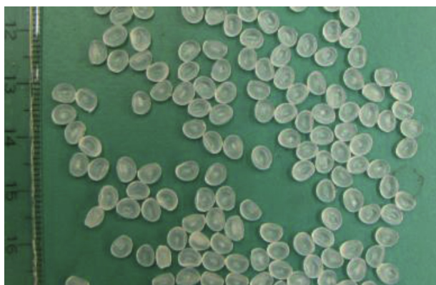
Fig. 2. Polypropylene (PP) granules used in the experiment.
