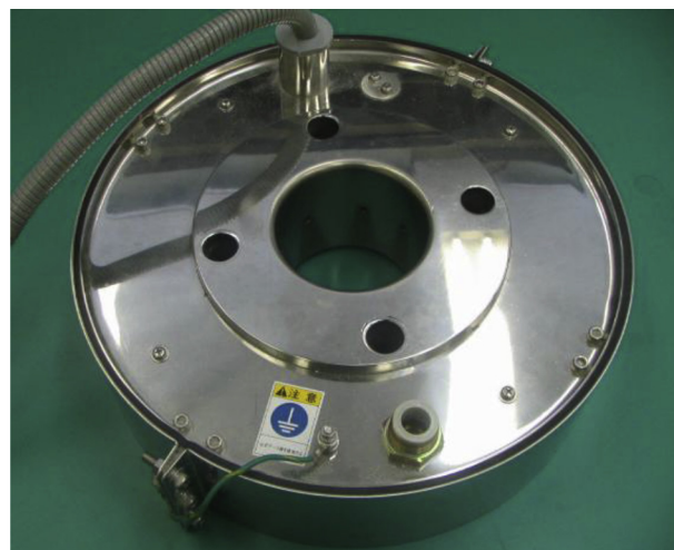
Fig. 3. Flange-type ionizer used in the experiment.
