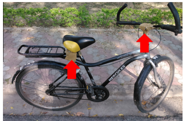
Fig. 1. Accelerometers installed on Bicycle.
