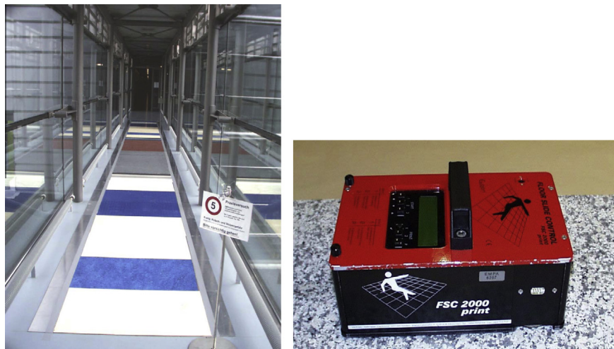
Fig. 1. Long-term experiment concerning the effectiveness and durability of anti-slip treatments (left) and the portable tribometer FSC 2000 used for friction measurements (right).
