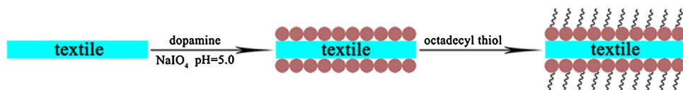
Fig. 1. Schematic illustration for fabrication of superhydrophobic coating on the textile.
