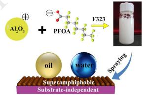
Robust superamphiphobic coating obtained from all-water-based spray can maintain liquid repellency after physical damages and long-term exposure to various harsh conditions, and has a self-repairing ability against chemical destruction.
