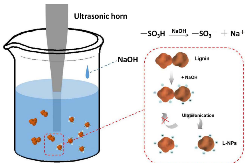
Scheme 1. Schematic illustration of synthesizing the L-NPs by the ultrasonic-assisted alkali method.
