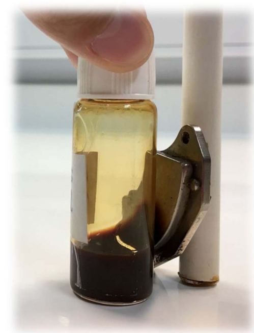
Fig. 1. MNPs response under the presence of a permanent magnet.
