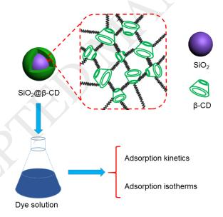
**Abstract**:  $\beta$ -cyclodextrin, a type of molecule with a cavity structure and large number of hydroxyl groups, has great potential in water treatment, attributing to its highly adsorption ability. In this work, silica nanoparticles coated with  $\beta$ -cyclodextrin (SiO<sub>2</sub>@ $\beta$ -CD) as adsorbent have been successfully synthesized via distillation-
