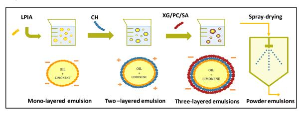
Schematic representation of the formation of multilayer emulsion system and spray-drying. LPIA: lupin protein isolate AluProt-CGNA, CH: Chitosan, XG: Xanthan Gum, PC: Pectin
