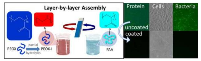
**Caption:** Layer-by-layer assemblies of partially hydrolysed poly(2-ethyl-2-oxazoline) (PEOX-I) and poly(acrylic acid) (PAA) provide for effective resistance against surface protein, cell and bacterial attachment.
