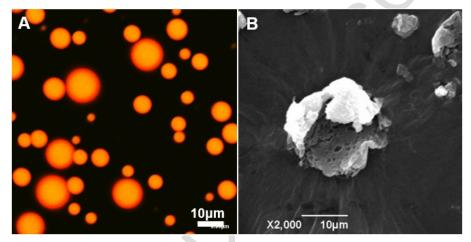
The core-shell structure of the limonene microencapsules was confirmed with CLSM (A) and SEM (B), which was prepared with 4 wt% limonene, 2 wt% zein and 1 wt% SC. The interior rough and porous shell was promising for the rate-limiting release of the core limonene.
