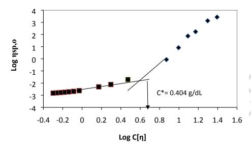
Zero shear specific viscosity versus volume concentration of *Delonix regia* polysaccharide
