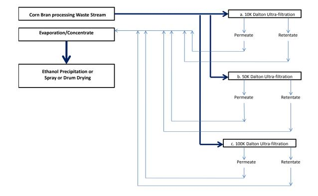
Scheme for ultrafiltration, evaporation and drying of corn bran processing waste stream
