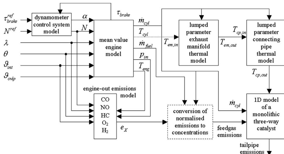
Fig. 1. Structure of the combined engine, emissions, exhaust and aftertreatment system model.
