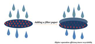
After adding of a superhydrophilic filter paper, the superhydrophobic membrane with flame retardency demonstrates better separation performances.
