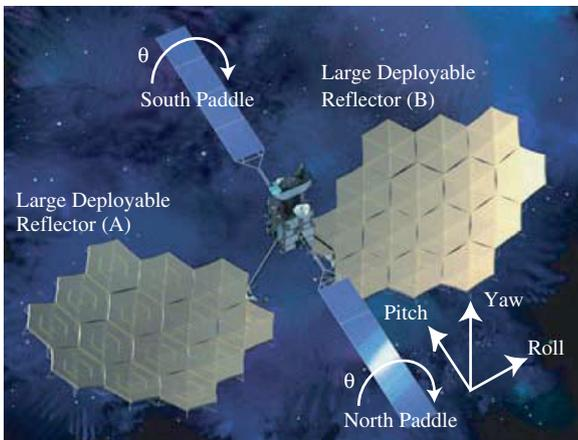
Fig. 1. Conceptual image of ETS-VIII and its coordinates.
