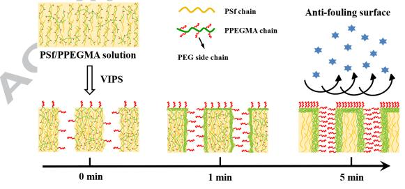
in situ PEGylated PSf membranes with increasing exposure time in humid air
