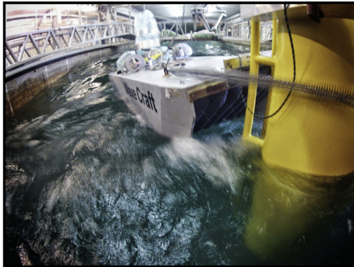
Fig. 1. The Wave Craft model-test and prototype in BCS mode. Courtesy of Umoë Mandal (UM).
