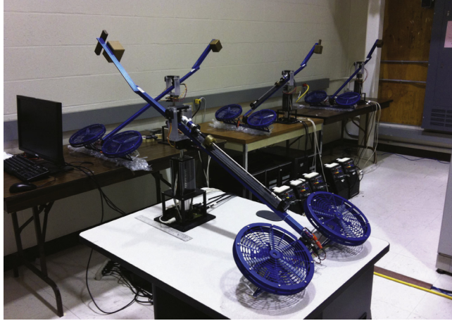
Fig. 2. The four three-DOF helicopter setup at UTIAS.
