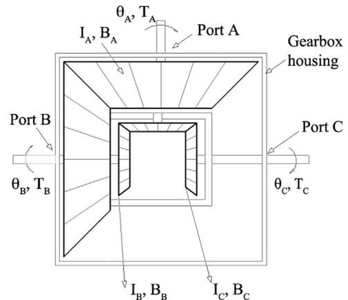
Fig. 1. Differential gearbox.
