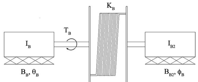
Fig. 2. Spring-mass-damper module attached to output B.
