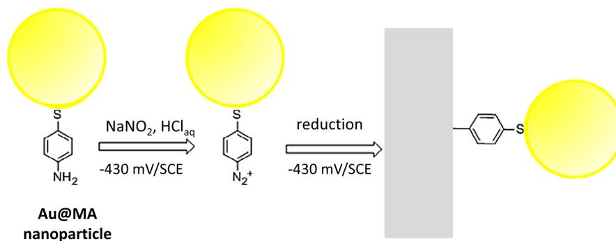
Scheme 1. Electrochemical grafting of Au@MA nanoparticles on a conductive substrate.
