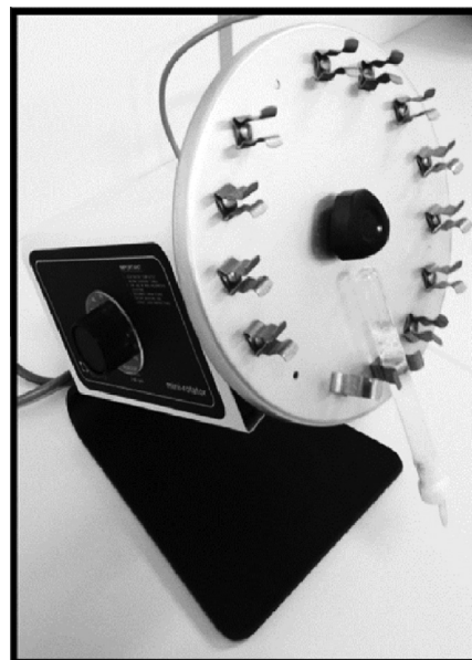
Fig. 1. The rotator with one test tube attached.
