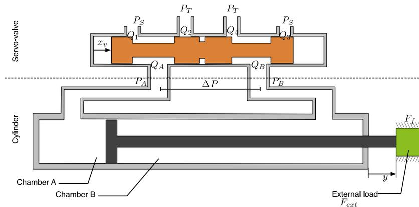
Fig. 1. Schematic diagram of the simplified SHA.
