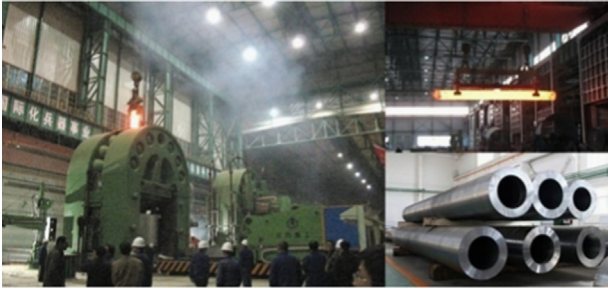
Fig. 1. The 360MN vertical extrusion press and the large-diameter thick-walled seamless tubes.
