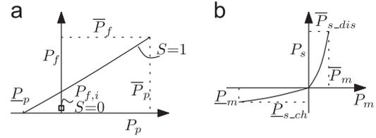
Fig. 2. Schematic cost functions of (a) engine and (b) electric machine and battery.
