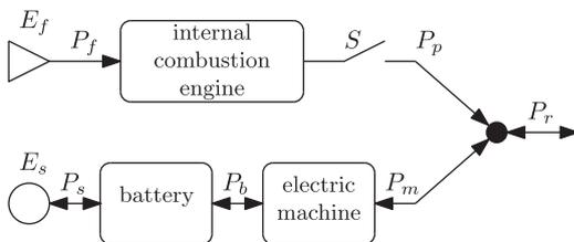
Fig. 1. Schematic overview of a hybrid drive train.
