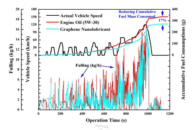
Novel approach of the graphene nanolubricant for energy saving via anti-friction/wear in automobile engines
