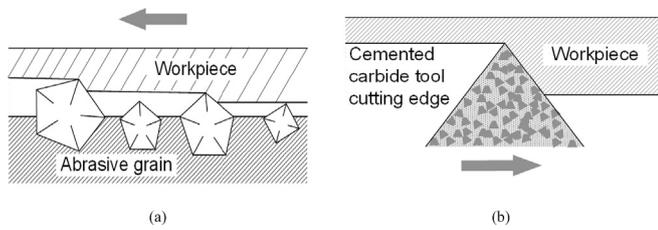
**Fig. 1.** Schematic illustration of material removal in (a) abrasive machining processes (where CBN composite is used as cutting tool); (b) chip-removal machining processes (where cemented carbide is used as cutting tool).
