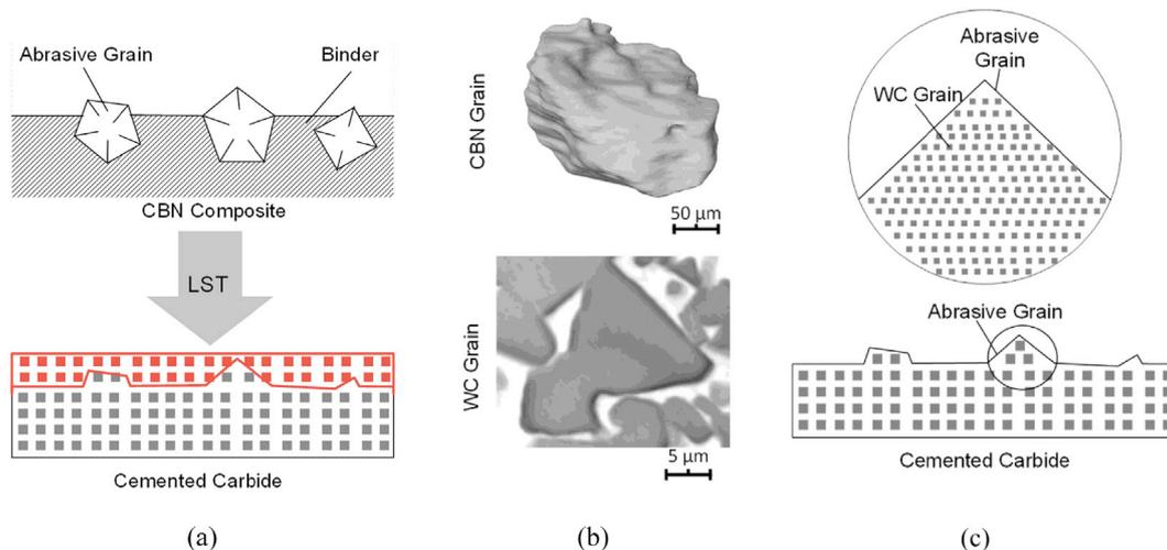
**Fig. 2.** (a) Schematic illustration of novel tool fabrication concept for honing processes; (b) grain size comparison between CBN grain and WC grain of the studied materials; (c) fabrication of abrasive grain with WC grains.
