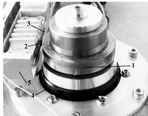
Fig. 2. Picture of tribo-couple: 1 – rotor with the coating, 2 – block of counter body, 3 – piezoelectric element, 4 – air-bearing, 5 – holder of piezoelement [12].
