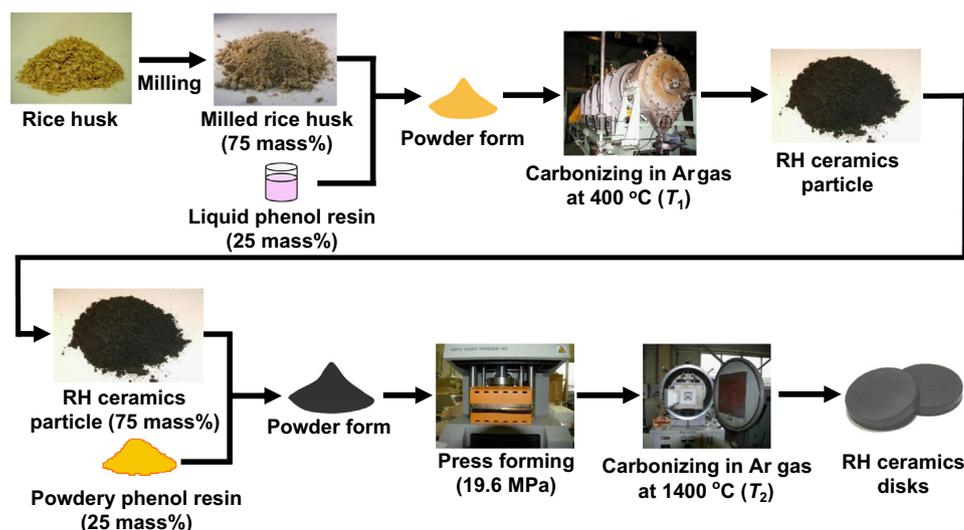
Fig. 1. Manufacturing process for RH ceramics.
