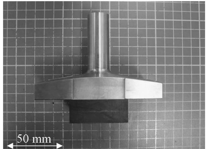
Fig. 1. The sample holder with a rubber block.
