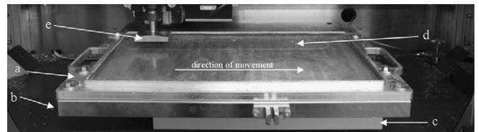
Fig. 2. Photograph of the new linear friction machine. The ice tray is bolted on the test table and the sample holder mounted on the moving part. (a) Tray, (b) aluminium table, (c) measuring platform, (d) milled track in ice, (e) rubber holder and rubber sample.
