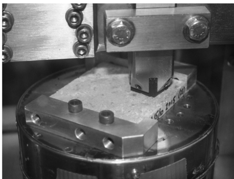
Fig. 2. Photograph of a tyre sample and a road material sample in contact.
