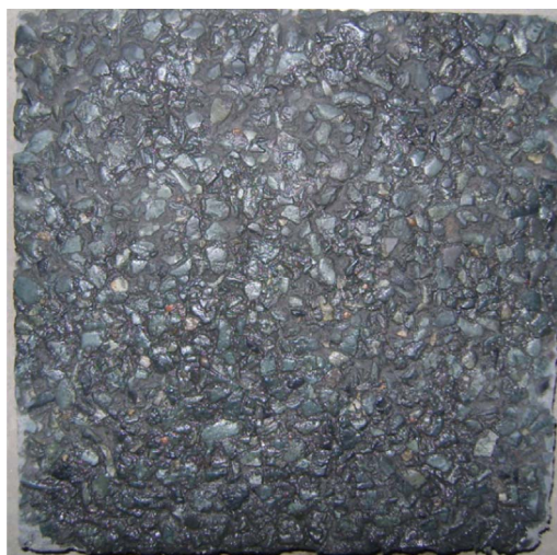
Fig. 3. Binder-free surface of SMA sample after polishing test.
