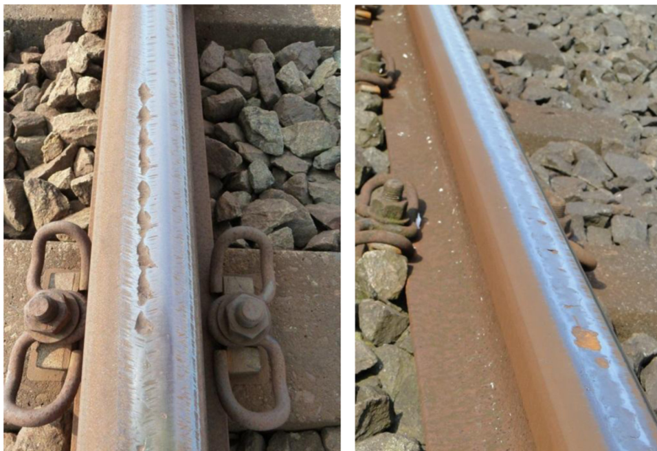
Fig. 1. Periodic spalling defects on heat-treated rail grade R370crHT/MHH.
