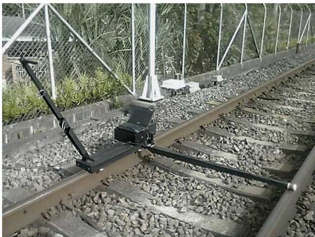
Fig. 1. Hand-pushed tribometer, TriboMetro FR-101 [10].
