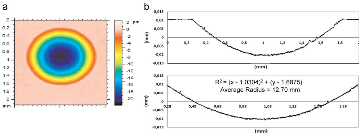
Fig.2. Profilometry analysis of the wear crater obtained with powder 100L and 0.2 N: (a) three-dimensional height data and (b) profile in the center of the crater and crater radius.
