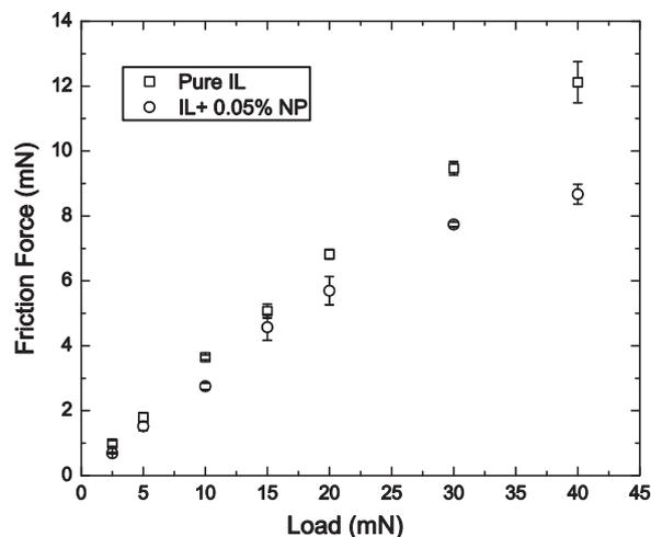
Fig. 1. The friction force as a function of load for simply and compositely lubricated conditions.
