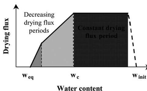
Fig. 1 – Cartoon of a standard drying curve.
