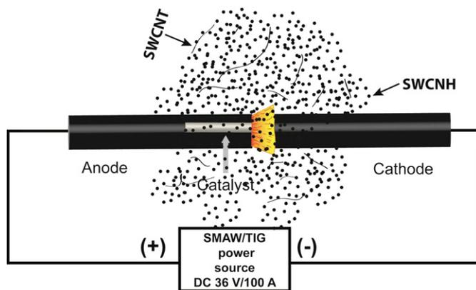
Fig. 1. Illustration of synthesis of NTNH hybrids by arc discharge technique.
