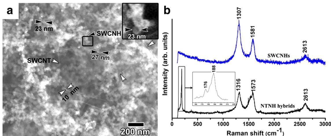
Fig. 2. (a) FE-SEM micrograph of thin SWCNT bundles with smaller aggregates of SWCNHs and (b) comparison of Raman spectra of NTNH hybrids and SWCNHs synthesized in similar conditions. All white and black arrows indicate the SWCNT and SWCNH, respectively.
