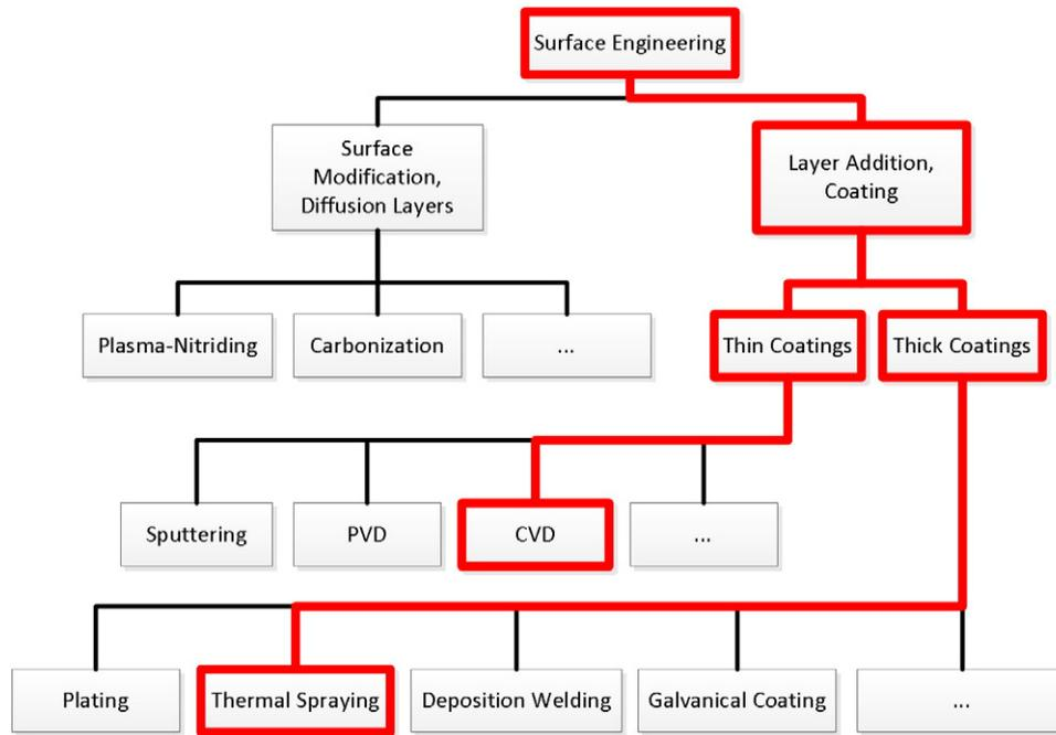
Fig. 1. Surface engineering technologies, highlighted: examined case examples.
