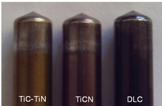
Fig. 2. Coated punches after forming Al 5083 with different grades of adhesive wear (light areas = penetration depth) [6].
