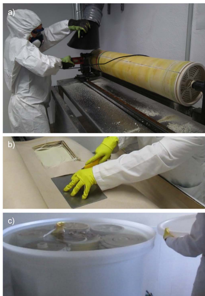
Fig. 1. End-of-life RO membrane autopsy: a) dissection of membrane module; b) extraction of membranes coupons and c) membrane storage.
