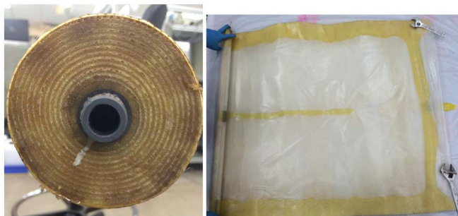
Fig. 1. Cross-sectional view of the spiral wound CTA membrane taken out of its module casing (left) and unwound (right).
