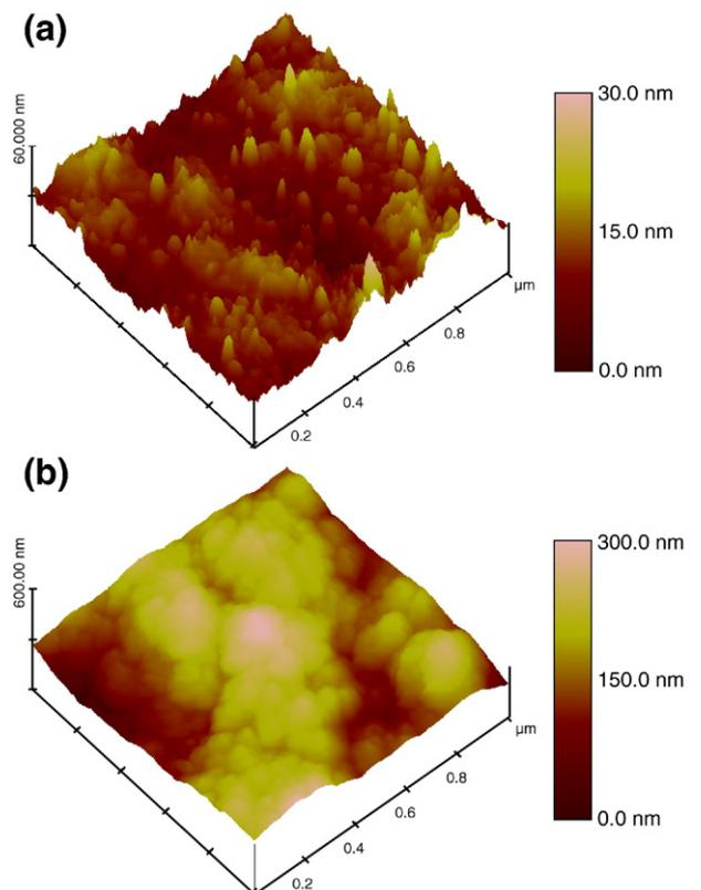
Fig. 2. AFM micrographs obtained on a  $1 \times 1 \mu\text{m}^2$  surface: (a) nucleation side of freestanding sample; (b) growth side of 4  $\mu\text{m}$ -thick NCD film.
