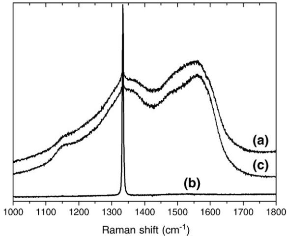
Fig. 1. Raman spectra acquired using a blue laser excitation wavelength (477 nm): (a) nucleation side of freestanding sample; (b) growth side of freestanding sample; (c) growth side of 4  $\mu\text{m}$ -thick NCD film.
