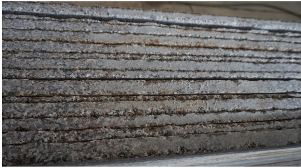
Fig. 2. The sawed slabs in marble frame saw machine.
